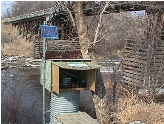
Clearwater River at Red Lake Falls automated river level gage
